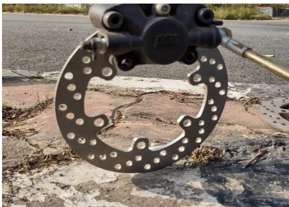
Figure 11 (b): Manufactured Rotor Plate
